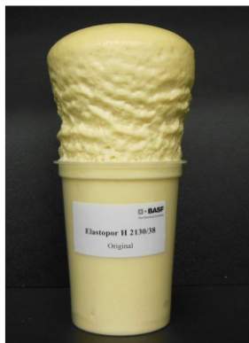
Figure 55: PU foam with ideal characteristics
