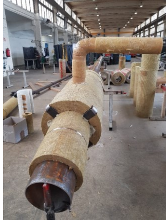
Figure: SMR - branch prefabricated in one unit
