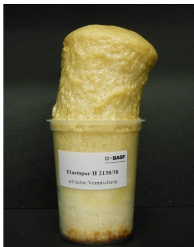
Figure 60: Poorly mixed PUR foam
