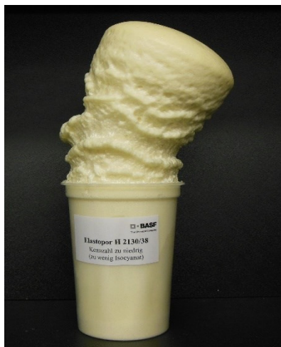
Figure 59: PUR foam with excess polyol
