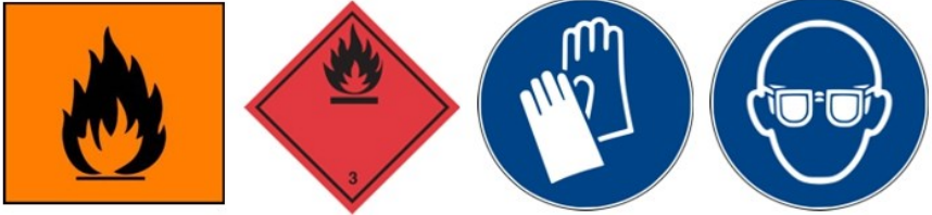
Figure 32, Warning and command signs for polyol
