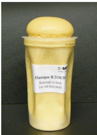
Figure 58: PUR foam with excess isocyanate
